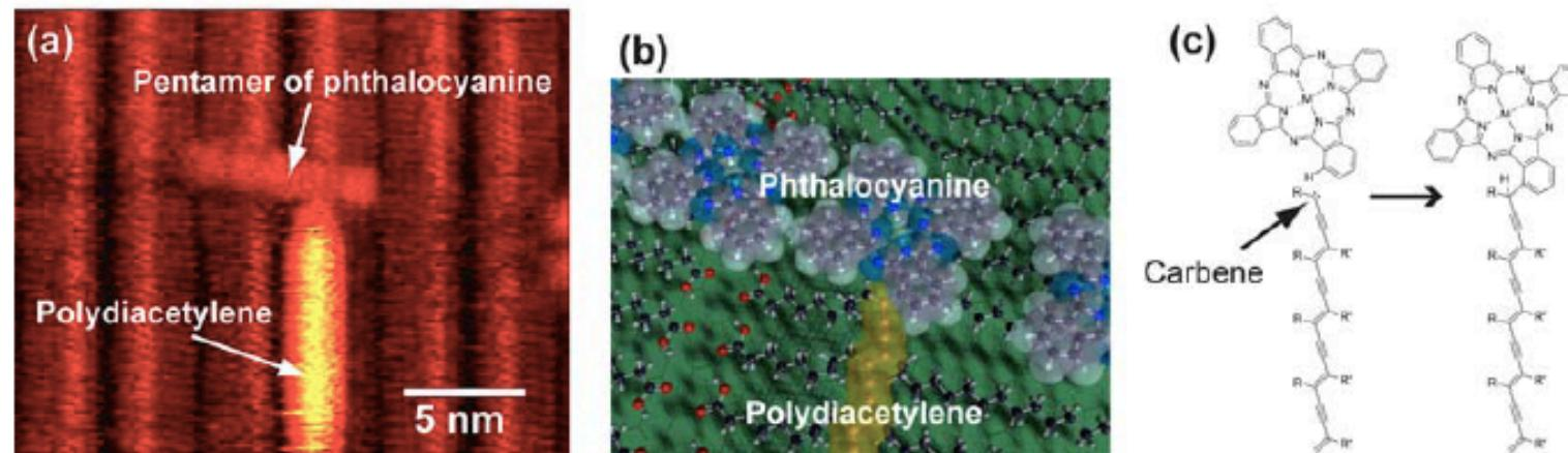
Figure. (a) STM image showing the connection of a single polydiacetylene chain to a single phthalocyanine molecule in a pentamer. (b) Structure model of the connection. (c) Insertion reaction of carbene at the end of polymer to a C–H bond of phthalocyanine.
