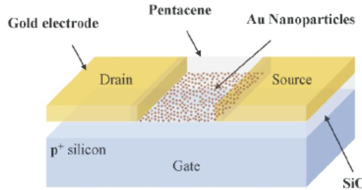
Input pulse rate determines the effective charge (balance between charging and leakage), controlling the conductance of the NOMFET.
