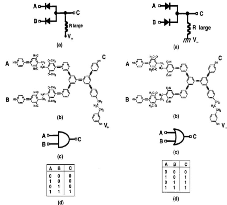
Figure 3.3: An early example of design of purely molecular AND and OR diode-resistor logic. Ellenbogen and Love [181].
