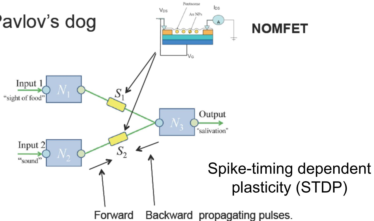
If the forward and backward pulses coincide in time, the voltage sum will exceed the threshold of the memristor synapse and cause the conductance to increase, until the sound of the bell can induce salivation on its own.
