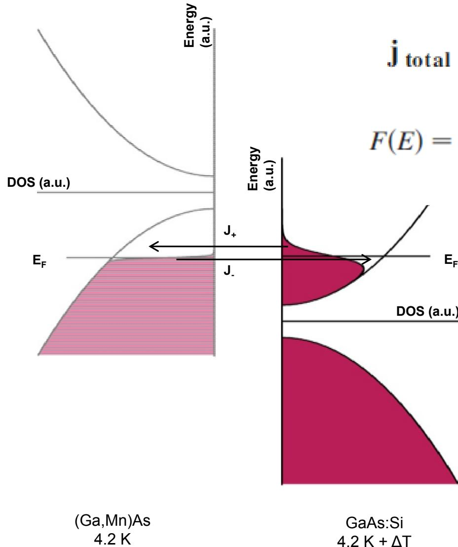
$$j_{\text{total}} = A \int_{E_{C,\text{GaAs:Si}}}^{E_{V,(Ga,Mn)\text{As}} - eV_{\text{th}}} F(E) dE$$
