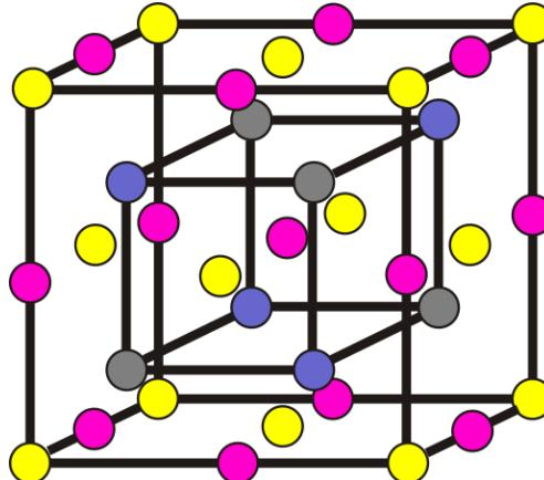
$\text{L2}_1$  structure  $\text{Ni}_2\text{MnSb}$
