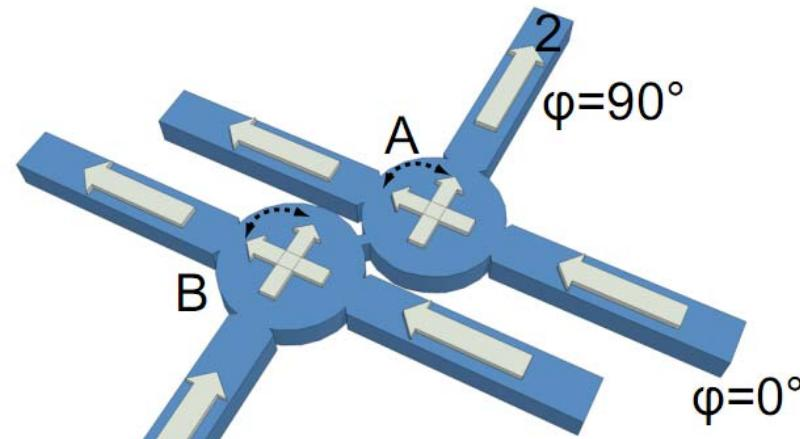
$$\begin{aligned} M \parallel 90^\circ &\rightarrow 0 \\ M \parallel 180^\circ &\rightarrow 1 \end{aligned}$$
