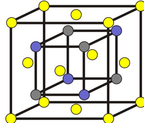
$\text{C1}_\text{b}$  structure  $\text{NiMnSb}$
