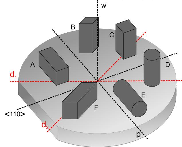
Silicon is an anisotropic material. Thus, a device characteristics depend on its orientation in the wafer.
