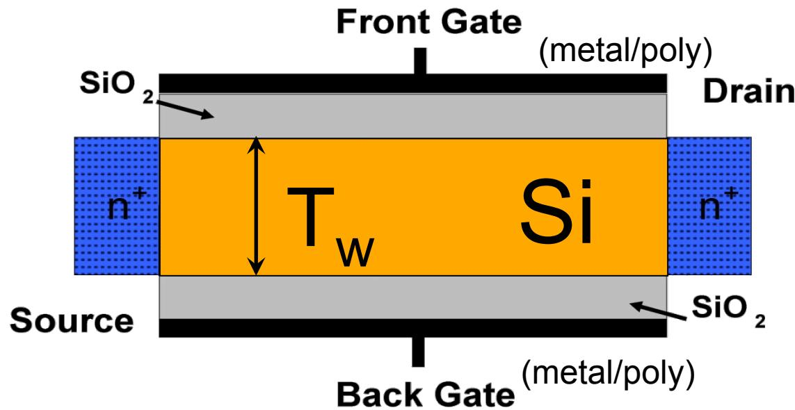
It is useful to improve the electrostatic control of the channel and avoid the Short Channel effects appearing in devices with Silicon channel length in the range of nanometers.
