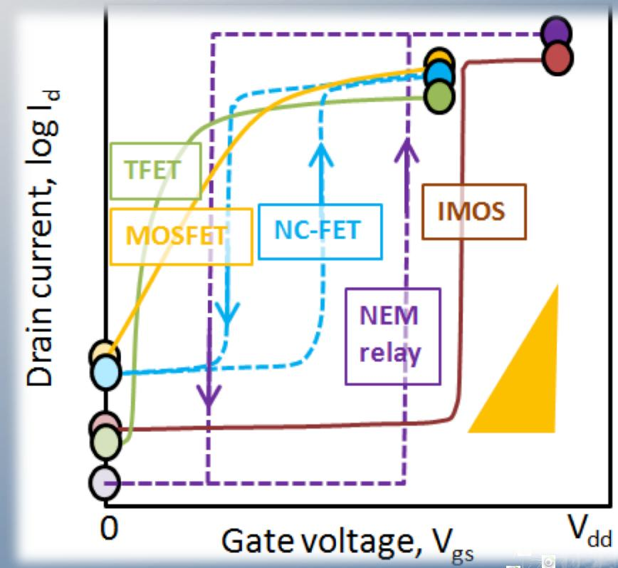
Tunnel FET is the most promising small swing switch for scaling the supply voltage and the energy per binary switching.
