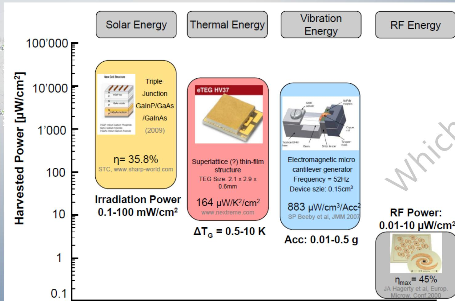
**No winning concept:** the analysis of the system specification defines the right type of harvester or combination of harvesters!
