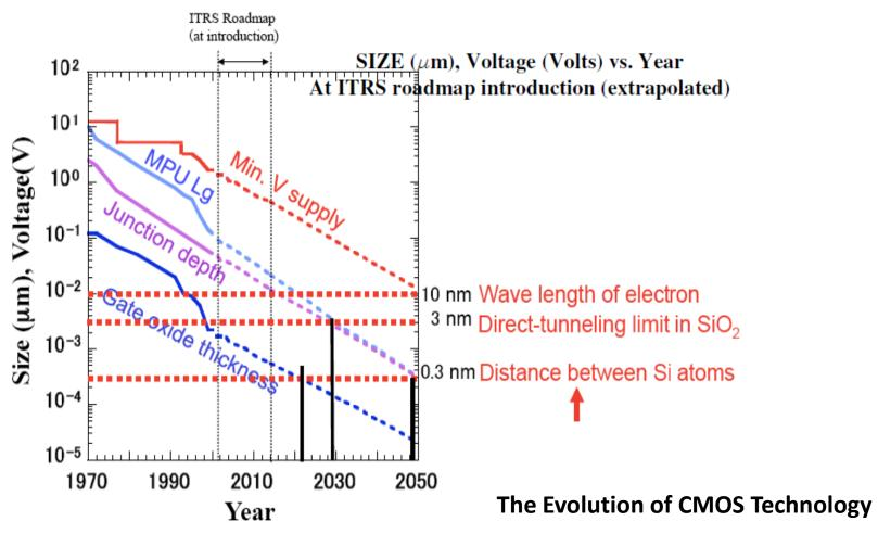
The minimum supply voltage, oxide thickness and junction depth. Comparison to basic physical limits – electron wavelength in conduction-band and distance between silicon atoms [Hiroshi, I.].
