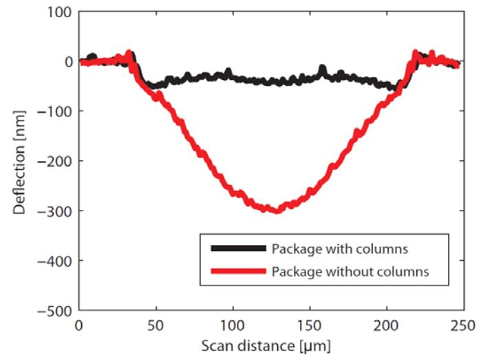
Deflection under 1 bar. Comparison between two square packages (180  $\mu\text{m}$  side length) with and without columns (4  $\mu\text{m}$  diameter). The deflection of the package with no columns is too large for many applications.
