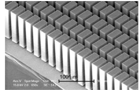
HAR fin-channel structure for microevaporator
