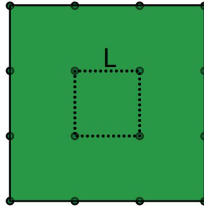
Thin-film package geometry consisting of a square plate with supporting columns
